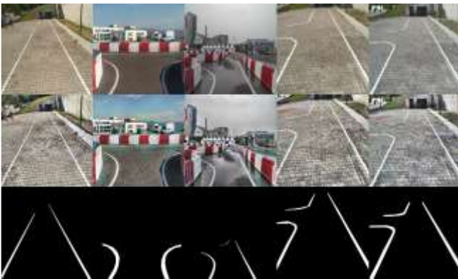
Fig. 1. Samples from the dataset showing the images with its corresponding masks.
