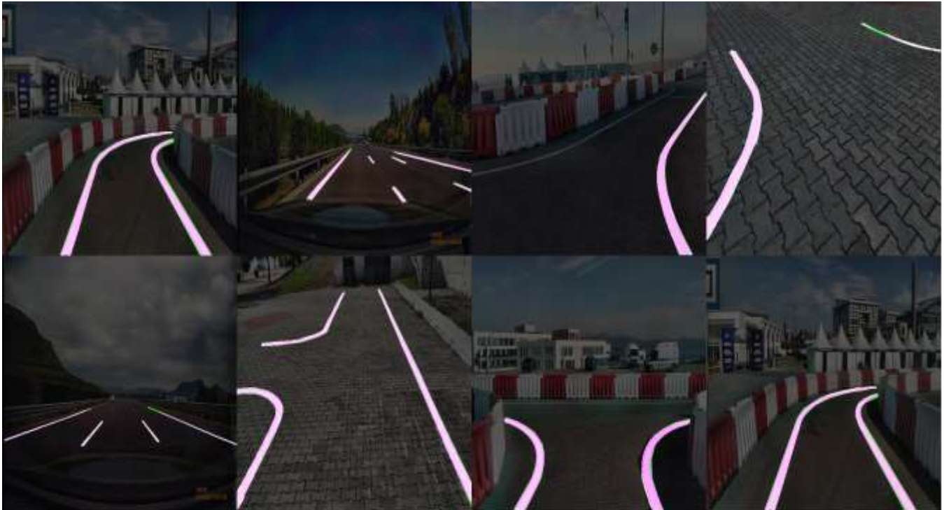
Fig. 2. Visual representation of the performance of the best-model on some testing data, where the green and magenta colors stand for the true lane and the predicted lane, respectively.
